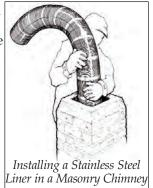
floor or ceiling joists, and at the roofline. There should be at least 2 inches of clearance between the chimney and floor joists or other combustible materials. Poor flashing between the chimney and the roof line can cause leaks and deterioration of chimney mortar.
